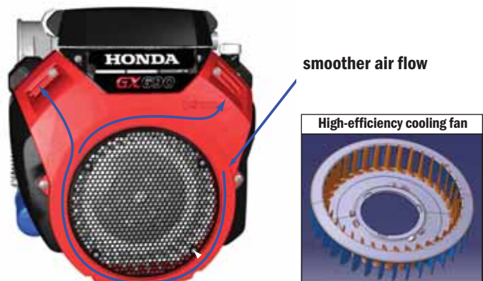
Cooling performance is improved while noise is reduced with the large diameter air intake, optimized 36-blade cooling fan and smooth scroll-shaped resin shroud.
